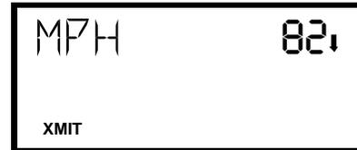
When Peak mode is ON, the PEAK icon appears on the display and the highest speed for each ball displays in the main window. The ball's roll-down speed displays in the upper right window.
