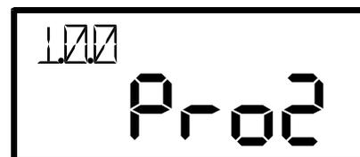
Briefly press the MENU key while the version is displayed to enter the **Fork Diagnostic**. The transmitter is turned on automatically and all directionality, filtering and special target processing is turned off so that any target moving in the range of 25-100 MPH will be displayed. A ringing tuning fork held in front of the radar should produce a steady speed display.
