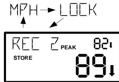
The most recently saved speed group shows first. Pressing the RECALL key briefly once more while the last speed group in the queue is displayed exits Recall Mode. Exit the recall queue at any time by pulling the trigger.
