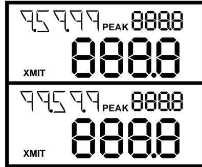
**Cosine Angle:** This setting is used to automatically correct speed readings for angle errors. It can be set in one degree increments in the range from 0 through 45 degrees. The default setting is 0 degrees. Refer to the Angle Errors section for more details.
