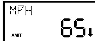
When Peak mode is ON, the PEAK icon appears on the display and the highest speed attained displays in the upper right window. The live vehicle speed displays in the main window.
