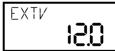
Briefly pressing the MENU key cycles the unit through the diagnostics. Pull the trigger at any time to exit Diagnostic Mode and return to Radar Mode.
