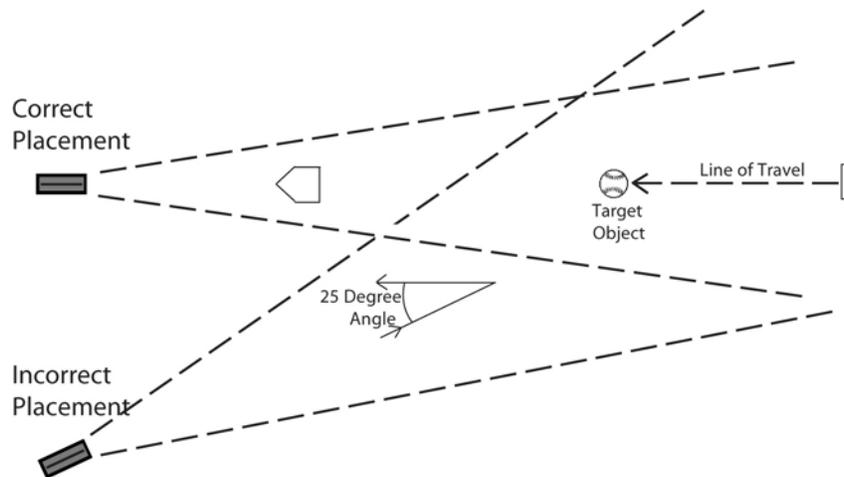
At slight angles the error is very small; however at larger angles, the error becomes substantial as the table below shows.
